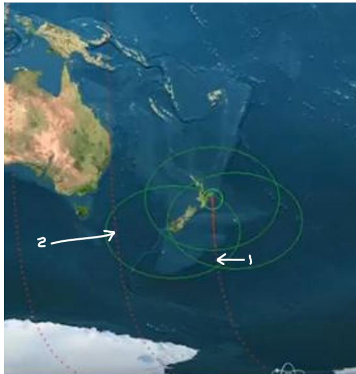
Figure 5. Rocket Lab Electron launch ground track. Awarua SGS acquires signal approximately 2 minutes after launch from Mahia (shown as 1) and approximately 100 minutes later (2). The third pass (far left of the map) is not visible from Awarua SGS.
