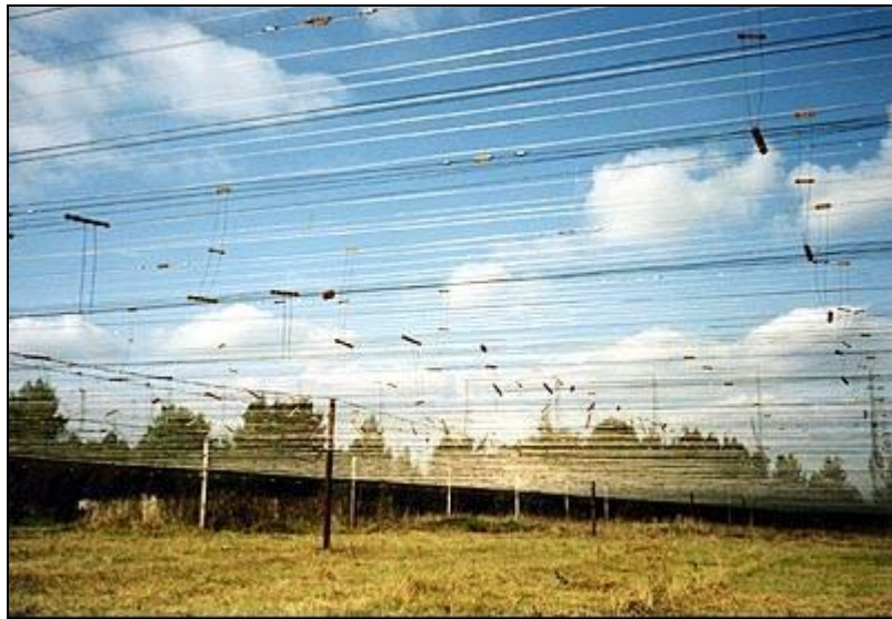
Figure 14. Pushchino VLF radio telescope consists of 16,384 wire dipoles, occupying 7ha.
